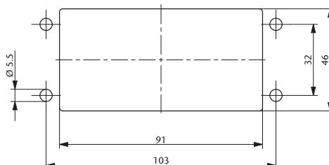
Torque for the frame's mounting screw: 2.5 – 3 Nm
