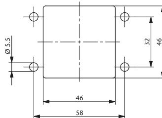
Torque for the frame's mounting screw: 2.5 – 3 Nm
