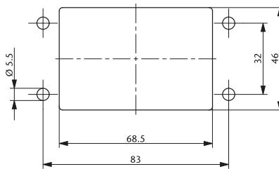
Torque for the frame's mounting screw: 2.5 – 3 Nm
